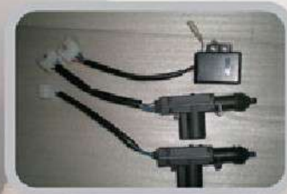
CENTRAL DOOR LOCK
